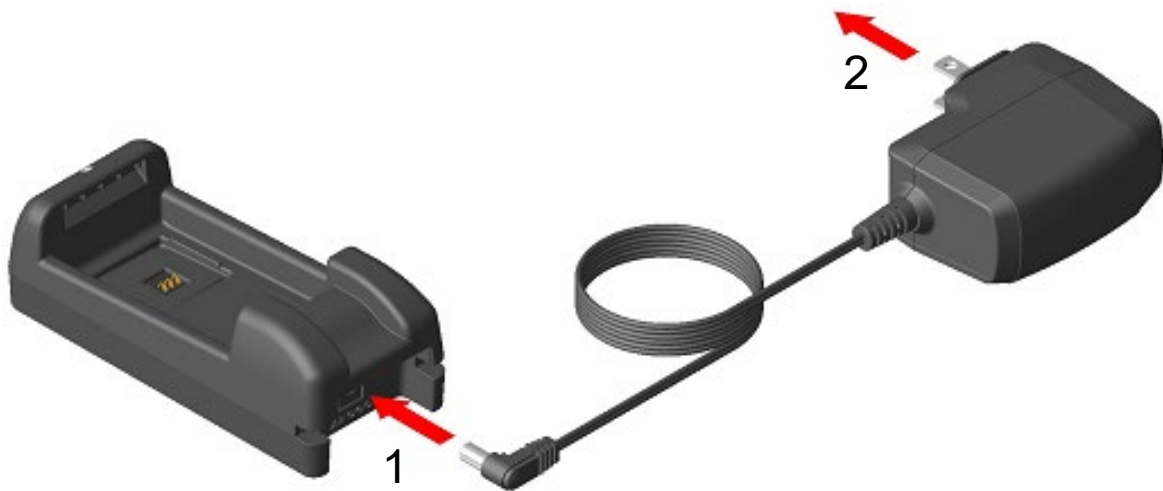
Figure 19-2 Battery Charger and AC Adapter Connection
