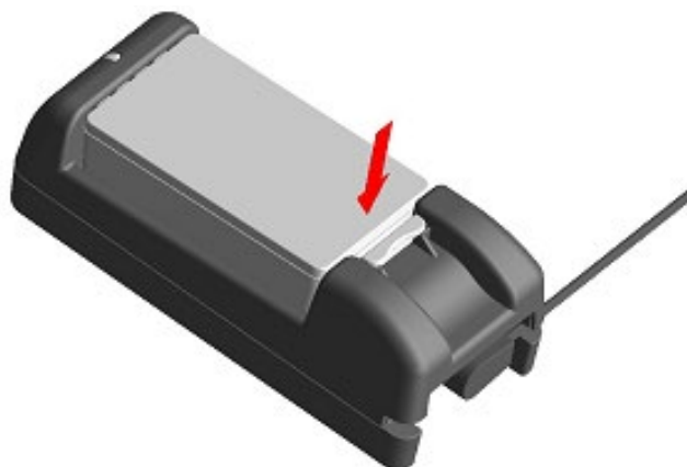
Figure 19-6 Installing Battery Pack (2)
